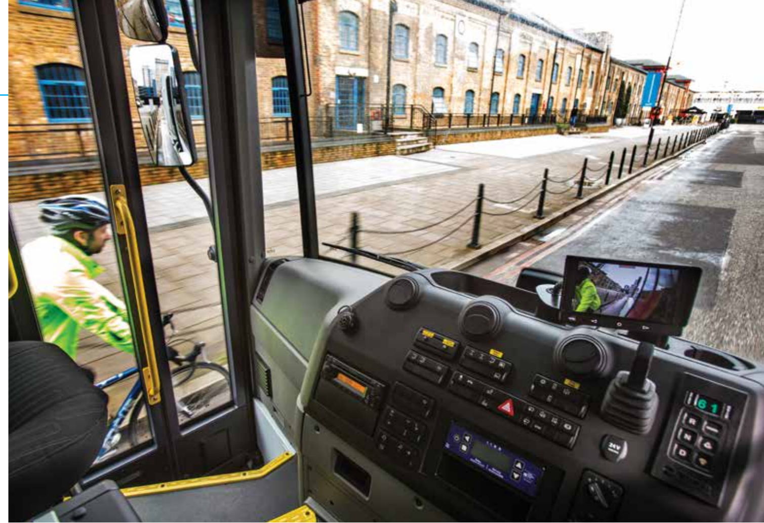
ABOVE: Mercedes-Benz Econic: Full-height nearside glazed scissor-type 'Bi-fold' door is standard
